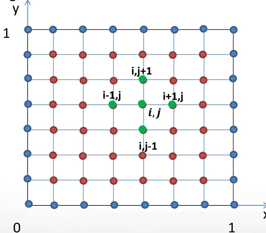
Discretize the domain along  $x$  and  $y$  using  $n$  internal points in each direction.
