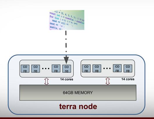
All modern computers have multiple processing cores (4 on average desktop). On terra, each **NODE** has 28 cores (two 14 core cpus) per node and at least 64GB of **SHARED** memory
