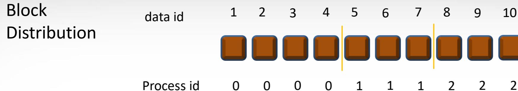
Data is partitioned into  $n$  contiguous parts, where  $n$  is equal to the number of processes. Each process will take one part of the data.
