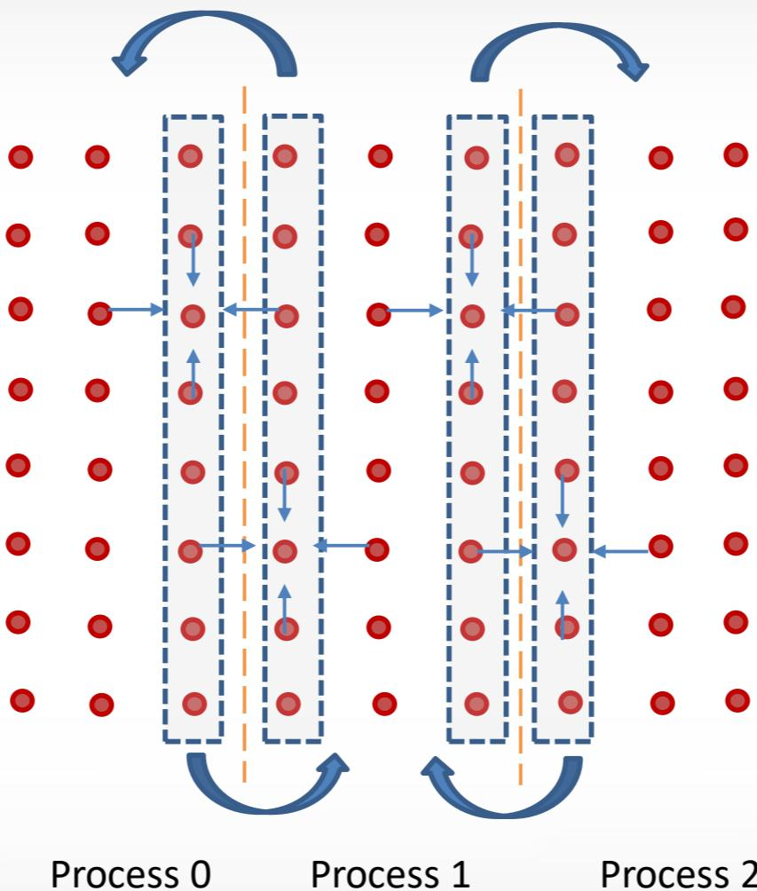
Border columns need to be copied into the memory space of the neighboring processes for the five-point stencil calculation. Same for row-wise decomposition.
