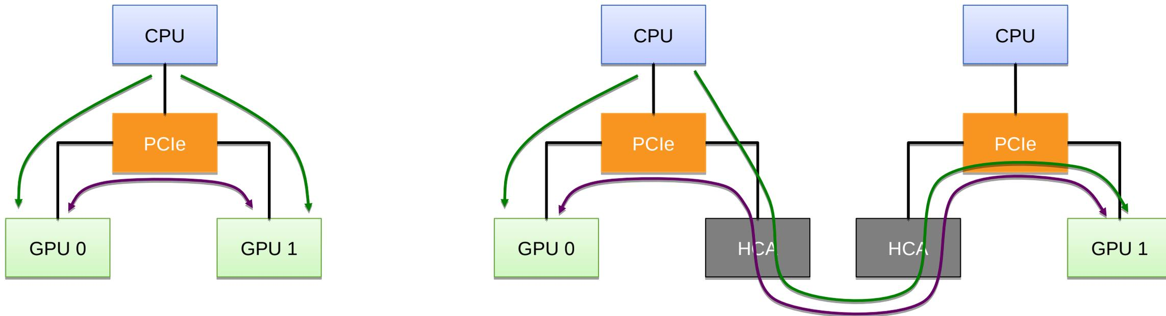
Completely transparent: All CUDA Apps see local and remote GPUs as if directly connected
