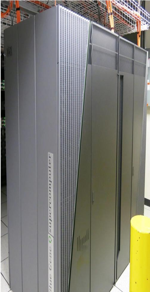
32768-core, 419 TFLOPS, Massively Parallel, interconnected in 5D Torus topology
