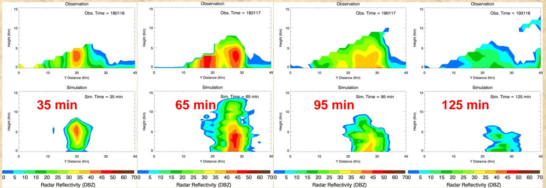
The simulated maximal radar reflectivity is 60.2 dBz, close to the observed 57.8 dBz;
