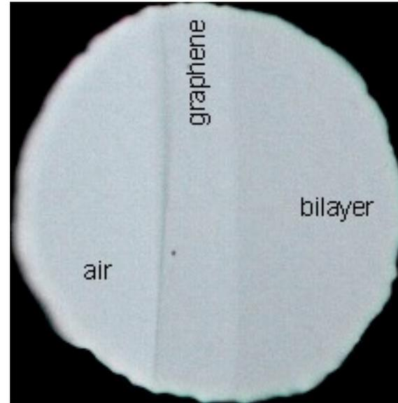
**Photograph of graphene in transmitted light. This one atom thick crystal can be seen with the naked eye because it absorbs approximately 2.3% of white light.**
