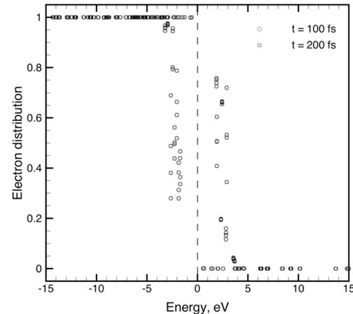
**Results shown are for 2-layer graphene: With nuclei frozen, electrons fail to equilibrate.**
