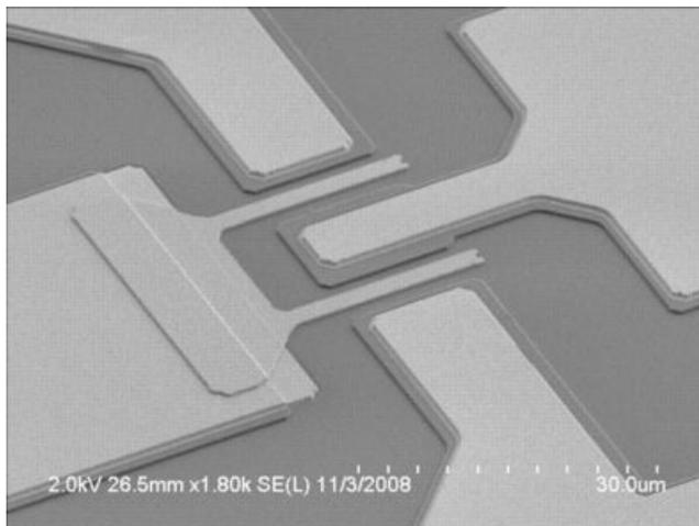
**HRL Laboratories demonstrated the first graphene field-effect transistors (FETs) using epitaxial graphene film operating in the radio frequency (RF) range.**
