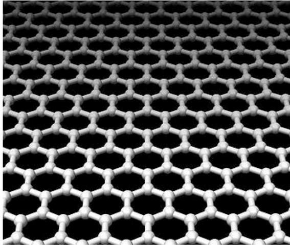
**Graphene is an atomic-scale honeycomb lattice made of carbon atoms. Measurements have shown that graphene has a breaking strength 200 times greater than steel, making it the strongest material ever tested.**
