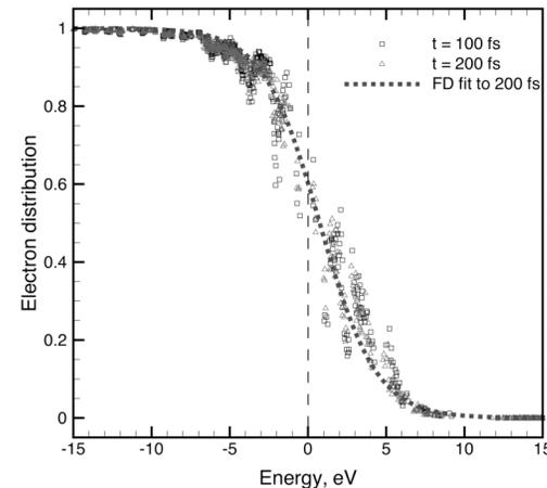
**With nuclei permitted to move, electrons equilibrate and form up into a Fermi-Dirac distribution.**
