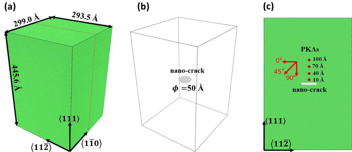
Configuration of simulation cell—Ni single crystal with a nanoscale crack
