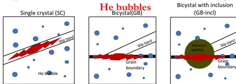
**Our goal: test this hypothesis via large-scale atomistic simulations of Ni with irradiation defects**
