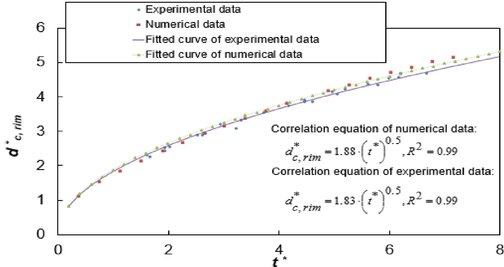
Numerical and experimental transient crown propagation curves
