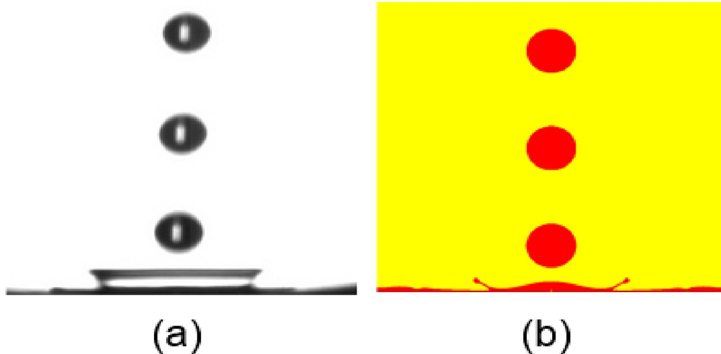
(a) Experimental and (b) numerical droplet-induced crown
