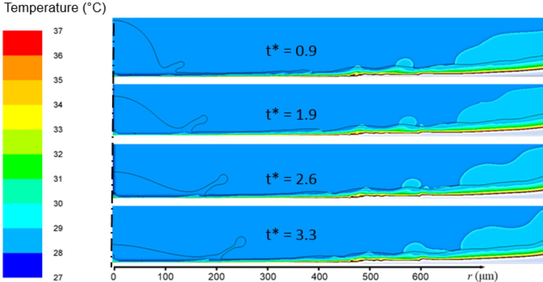
Instantaneous temperature field at a heat flux of  $3 \text{ W/cm}^2$  and  $We = 280$
