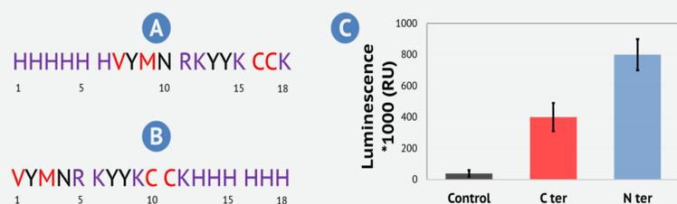
Fig.2: Chemical structures of HexaHis affinity tagged NFO4 at (A) N-terminus (N-ter, blue), (B) C-terminus (C-ter, red). (C) Influence of the aptamer modifications when immobilized at 1000 µg L<sup>-1</sup> on OTA detection. The control sample is the luminescence emitted with OTA-HRP without NFO4 peptide. Nter NFO4 binds more specifically to OTA as opposed to Cter NFO4.[1] Redrawn from Ref [1]
