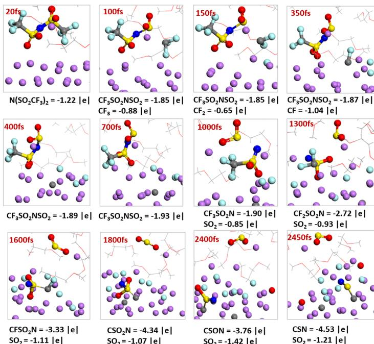
multiple electrolyte decomposition reactions at the surface of the Li metal anode identified by AIMD simulations
