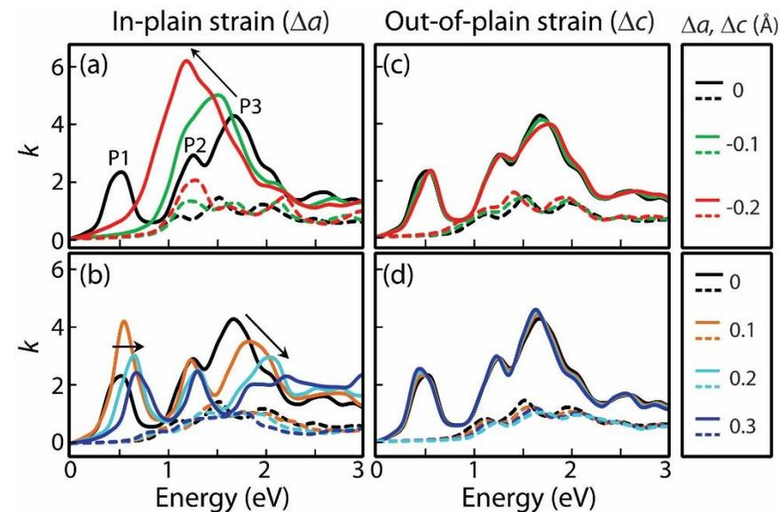
Imaginary part of refractive index ( $k$ ) under varying degrees of lattice strain
