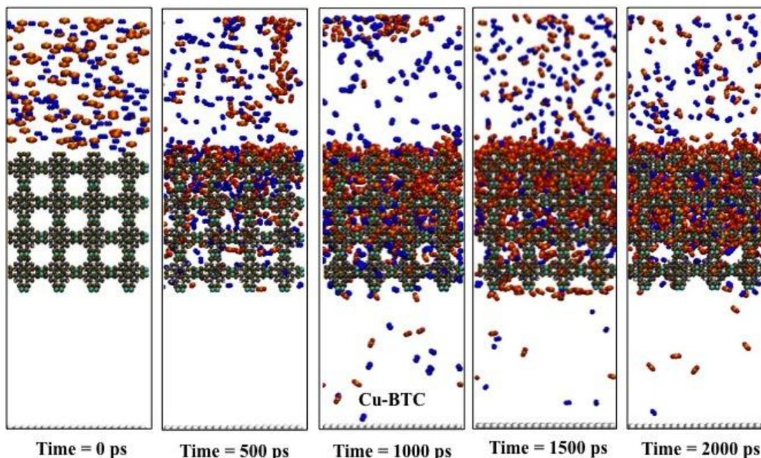
Once an efficient material has been identified for gas storage or separations, a membrane is fabricated. The mixture of gases passes through the membrane and selectively one of the gases is trapped. Here we simulate membrane operation at the actual pressure and temperature conditions
