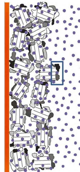
interfacial reactions generate a multicomponent solid-electrolyte interphase (SEI) film. Its properties are key for the battery lifetime
